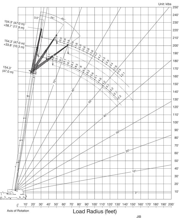
NOTE: Jib geometry shown are for unloaded condition and machine standing level on firm supporting surface.
