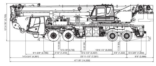
Note: Dimension is with boom angle at -0.4 degree.
