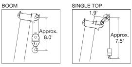
NOTE: Boom geometry shown are for unloaded condition and machine standing level on firm supporting surface.
