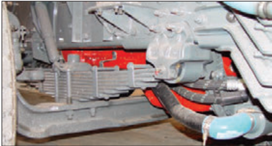
Spring front suspension w/air ride rear suspension provides a comfortable ride at 65 m.p.h. (105 Km/h)
